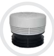
The AAV32-63 AAV provides a universal connector for 32mm, 40mm 50mm and 63mm waste pipes, and the AAV70-110 32mm is an ideal air admittance valve for 70mm, 75m, 90mm and 110mm soil pipe systems.
