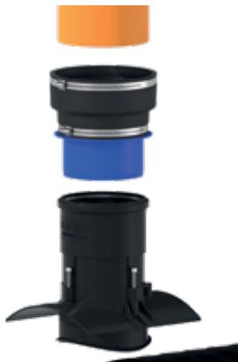
The PA Saddle will accept a 160mm PVC lateral pipe as standard, however, the saddle can be made universal by adding a Lateral Pipe Adaptor. The adaptor can be installed into the saddle which can branch off to fit a different material DN150 pipe or a smaller DN100 pipe.
